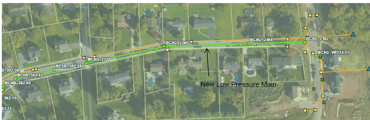
Figure 1: Low Pressure Sewer Extension Layout
